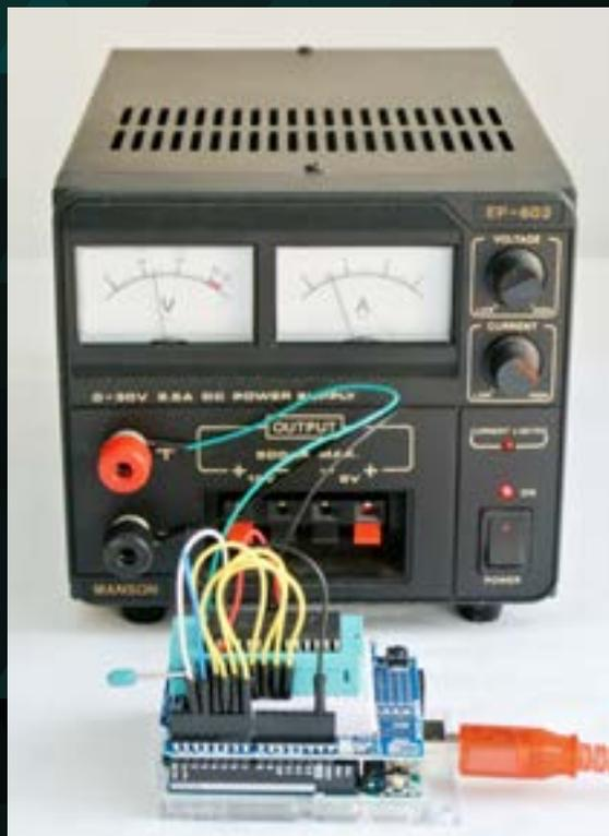
Verification of PIC16C57C using Arduino
