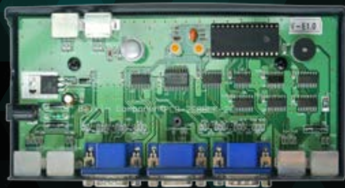
Belkin E Series OmniView 2-Port KVM Switch Internals
